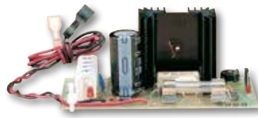
AD12612 Auxiliary Power Supply/Battery Charger
