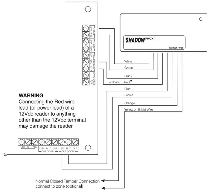
**NOTE:** Only use the +12V power supply when using ShadowProx Readers.
