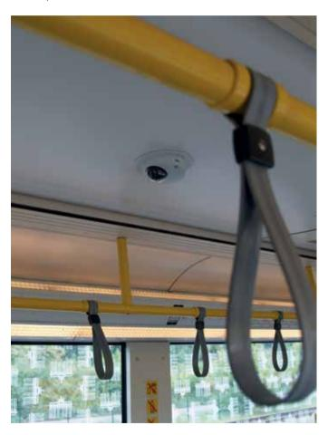
Figure 2: A camera with edge storage in an onboard installation.
