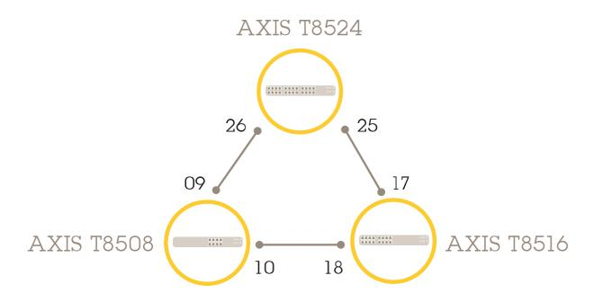
To create a redundant link on each switch's web page:
