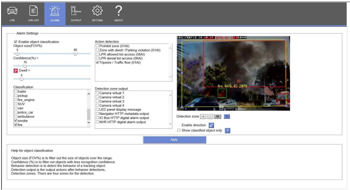
**Warning:** This technology uses AI image detection technology to detect smoke or fire. Rain, blocked camera or AI detection rate may cause AI technology to trigger false alarms or not triggering an alarm. Do not use this device as fire safety equipment smoke detector and fire detector.
