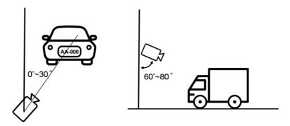
The angle of the license plate cannot exceed 15 degrees. To increase recognition rate, please rotate the camera to the same angle of the license plate.
