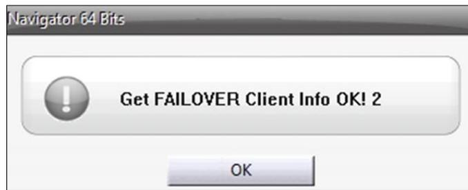
To test this function, for example, the Navigator recorders (failover clients) suddenly power down at 13:57:00, failover server will start recording selected channel until failover clients are recovered.
