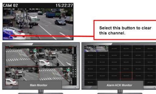
**Note:** To enable the acknowledgement function, click **Alarm ACK** in the alarm output management list.
