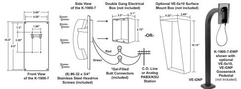
\* Note: The gel-filled (water-tight) butt connectors are designed for insulating displacement on 19-26 gauge wire with a maximum insulation of 0.082 inches. Cut off stripped wire ends before terminating.
