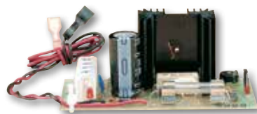
AD12612 Auxiliary Power Supply/Battery Charger
