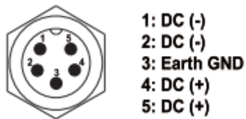
Figure 7: Redundant Power Supply Connector Pin-Out
