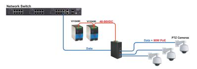
Multiple Vi10480 can share current to power a wide variety high PoE power PoE switches or Midspans. Also can be used as redundant power supply.
