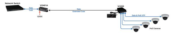
The Vi3205 can receive data over extended distance Coax up to 3,000 ft. at 100Mbps and power 4 PoE cameras using local power supplies.
