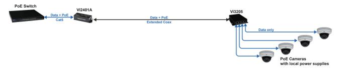
The Vi3205 can receive data and PoE power for powering itself over extended distance Coax up to 3,000 ft. at 100Mbps. The cameras use local power supplies.
