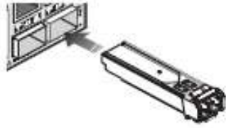
Figure 12: Inserting an SFP Transceiver into a Slot
