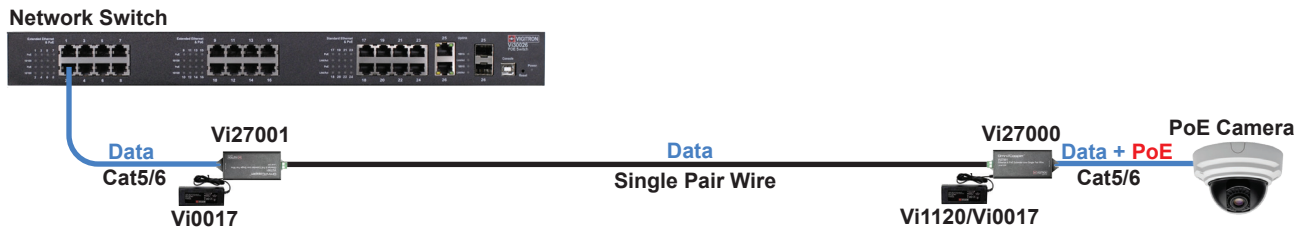
Both the Vi27001 and the Vi27000 can use local power supplies to power themselves and provide PoE to the IP camera.
