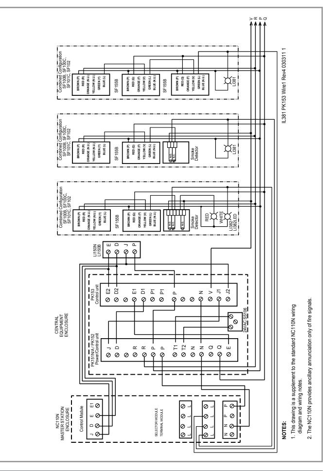
Figure 17—PK153 Wiring Diagram
