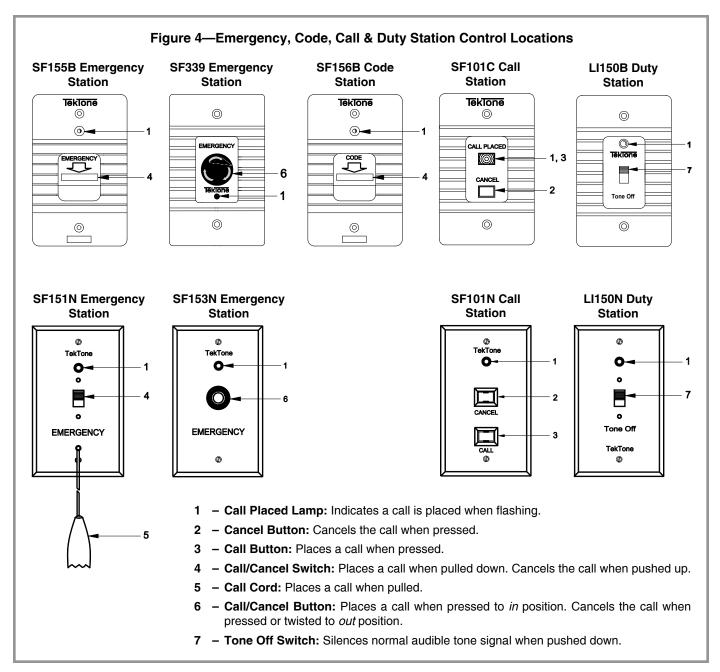
*Improper Operation:* If the call station does not operate as described, contact qualified service personnel. There are no user serviceable parts on the SF155B, SF339, SF151N, SF153N Emergency Stations or the SF156B Code Station.
