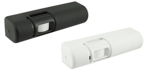
SDC's MD-31D series motion sensors are passive infrared detector specifically designed for request-to-exit applications. The coverage field is internally pointable. When angled 14 degrees down, coverage may be 5' x 6' at 7' feet high for 10' x 12' at 15' high. The MD-31D projects a wrap around "U" pattern down and away from the door to inhibit tampering.
