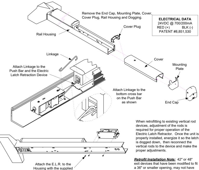
Replace Housing Cover, Cover with Plug, End Cap and the End Cap Cover.
