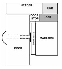
Sample Stop Filler Plate (SFP) and Universal Header Bracket (UHB) combination
