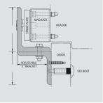
Accessories are available in a clear aluminum or black anodized finish. Verify length of magnetic lock before ordering mounting accessories.
