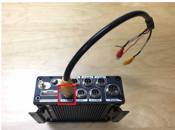
3. XDR Rear – Connect EX4-PIG to AV-OUT port on XDR for video out connection to monitor. May need BNC to RCA converter
