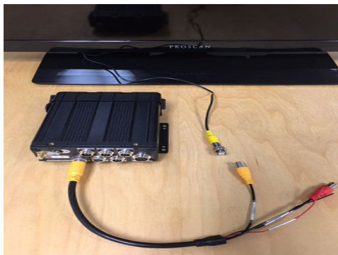
4. XDR Rear – Connect EX4-PIG to RCA video connection to monitor to monitor
