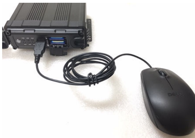
2. Connect USB mouse to XDR for programming
