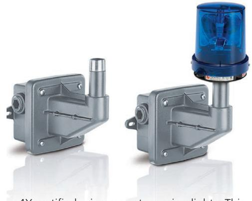
Model LSWB wall mounting kit is designed for use with Federal Signal's Type 4X certified, pipe mount warning lights. This kit features a 1/2-inch NPT pipe connection and is supplied with a surface mount weatherproof backbox.
