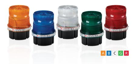
Model FB2LED is a multi-pattern LED available in five colors and features Federal Signal's patented Power Select™ technology. Power Select™ allows a user to select one of three flash patterns (60FPM, 120FPM or steady) without having to open the device. Units will come pre-set at 60FPM, but users can select one of the other two flash patterns by following a sequence when power is applied to the unit.
