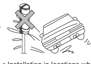
• Installation in locations where the device may be splashed by dirty water or direct sea spray.
