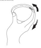
(7) When sensor unit is locked, tighten the locking screw.
