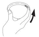
(6) When sensor unit is detached, hold it and slide release lever as illustrated
