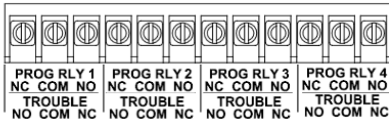
Figure 12. Relay Output Wiring
