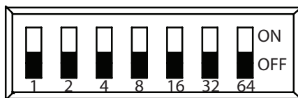
FIGURE 13: Enlarged View of PAD Device with Dip Switch Setting Unaddressed
