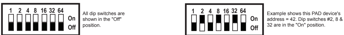
Figure 2. Examples of PAD Device Showing Default Dip Switch Setting (Unaddressed) & Addressed PAD Device
