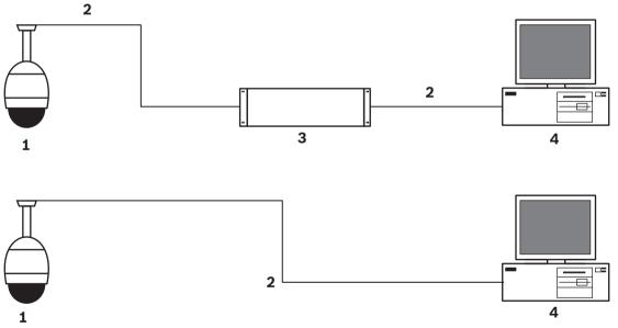
Figure 11.1: AUTODOME IP System Config
