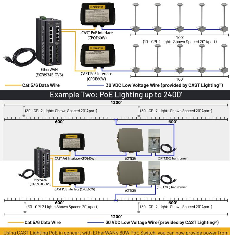
Using CAST Lighting PoE in concert with EtherWAN's 60W PoE Switch, you can now provide power from ONE switch. Power low voltage lights, cameras, access control, perimeter intrusion and tie into the network with one piece of equipment.
