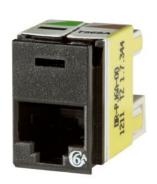
Clarity 6A patch panel jacks, rear load into patch panels and exceed Category 6a component specifications. Rear load positive latch design, secures mounting of the jack into the patch panel. Universal T568A/B wiring label and tapered wiring towers simplify termination.
