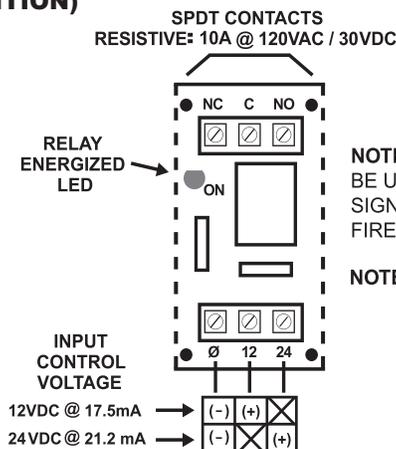
NOTE: INPUT POWER SUPPLY SHOULD BE UL LISTED FOR FIRE PROTECTION SIGNALING SYSTEMS WHEN USED IN FIRE ALARM APPLICATIONS
