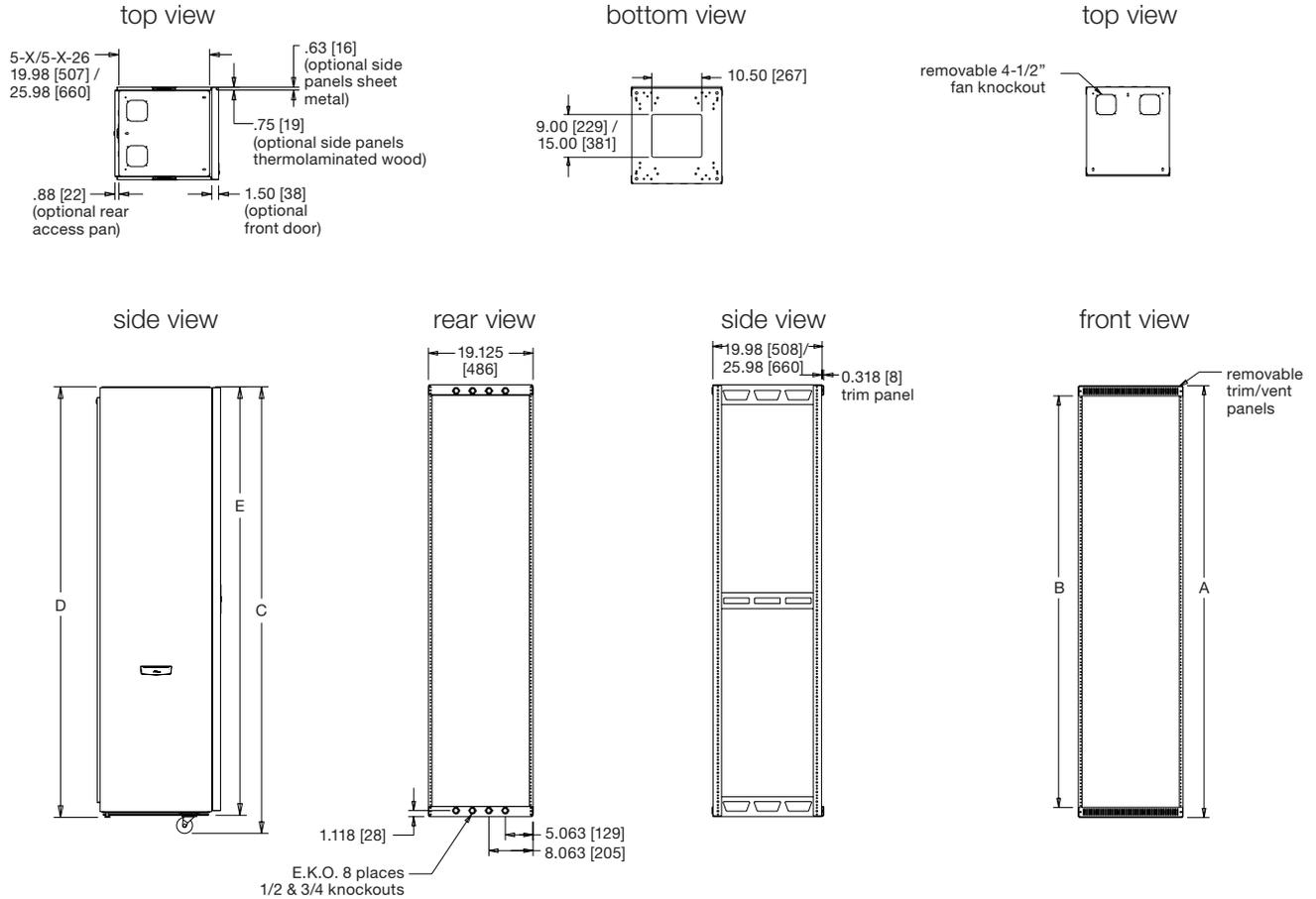
Note: Some dimensions are given for both 5-X and 5-X-26 in the form (5-X / 5-X-26)
