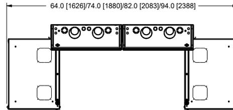
.25 [6] MIN. DISTANCE REQUIRED BETWEEN DWR'S USING ZERO CLEARANCE LATCHES MAP P/N: DWRSR-ZL
