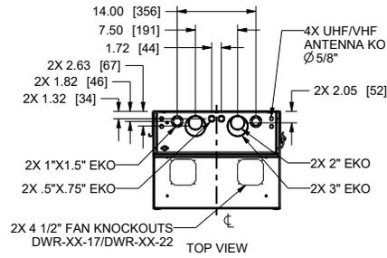
KNOCKOUTS PICTURED IN TOP VIEW ARE ALSO LOCATED ON THE BOTTOM VIEW
