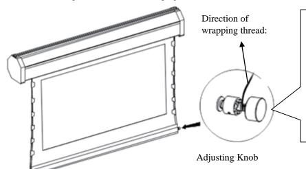
Adjustment method: Pull out the adjusting knob and rotate it to tighten or loosen tension string. The direction to tighten/loosen the string will depend on the direction of the wrapping thread.
