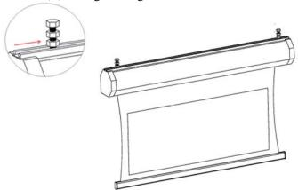
2. Slide the **Extruded Hanging Bracket (D)** through the rail located below the slide channel until it meets with the top of the **Bolt (B)** and slightly secure the lug-nuts located on the top & bottom of the bolt to attach the bracket.
