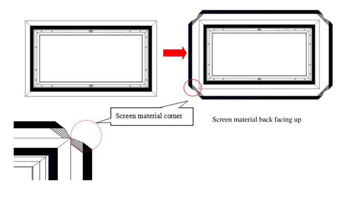
3. After all of the corners of the frame have been properly aligned, attach the material to the frame in the following order  $A \rightarrow B \rightarrow C \rightarrow D$  (see instructions below for details).
