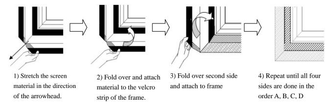
4. After all four corners have been attached; please check whether the frame corners are wrapped by the screen material. If not, please loosen the velcro connection and repeat the above steps so the frame is not exposed.
