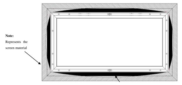
**Note**: The black shaded part represents the velcro on the frame. That Velcro end will ultimately attach with the other velcro end on the screen material.
