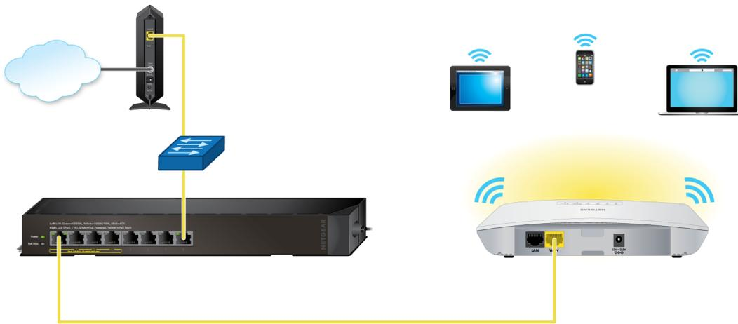
Figure 6. Set up the access point with a connection to your network
