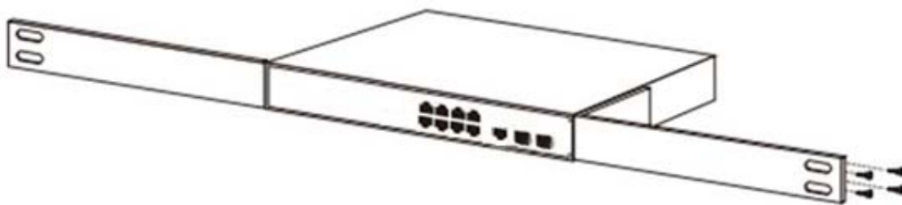
Figure 5 - Bracket Installation
