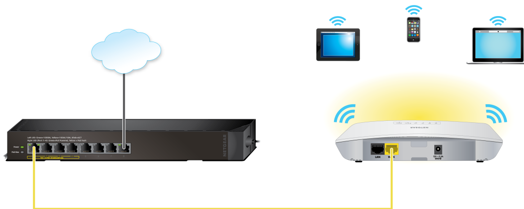
Figure 4. Set up the access point with a PoE connection to your network
