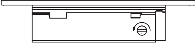
Fig. 1 Fail Safe = screw fully counter clockwise
