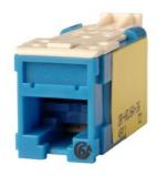
Clarity Cat 5E, CAT6 & CAT6A High Density Jack, ETL verified to TIA Category 5E, 6 & 6A component specification. Rear-loading, 180° exit, 8 position. Quick and easy lacing cap termination. Universal T568A/B wiring label. Center tuned to Clarity 5E patch cords for optimum performance.
