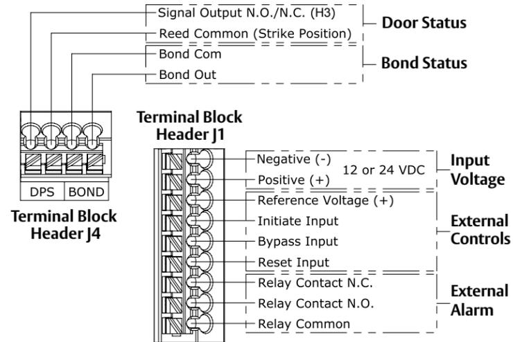
Diagram 26 Typical system wiring
