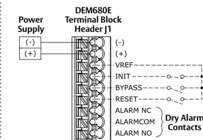
"(+)" and "VREF" Terminals are internally bussed to provide reference (+) voltage external control use.
