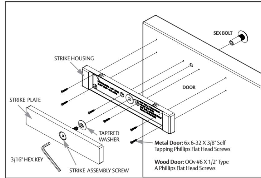
**Diagram 14** Strike assembly installed – section view
