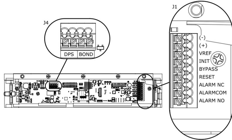
Diagram 25 Terminal pin-out diagram
