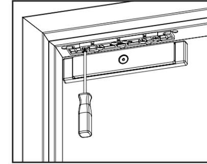
**Diagram 19** Installing the final mounting screws
