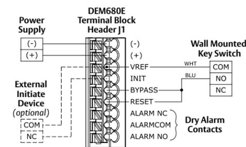
Diagram 28 Typical system wiring with external controls
