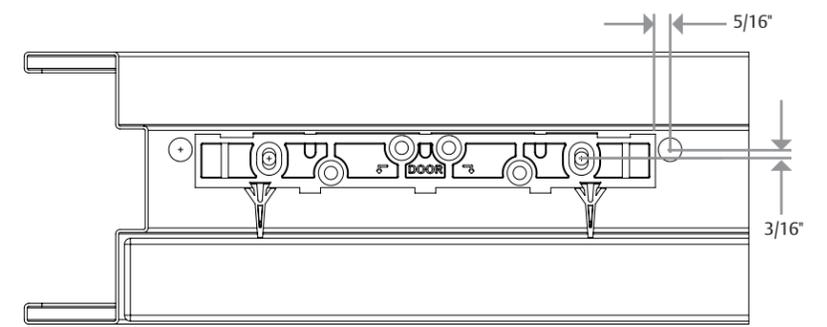
**Diagram 7** Drilling the bracket mounting holes
