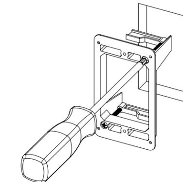
**Diagram 23** Installing the key switch
