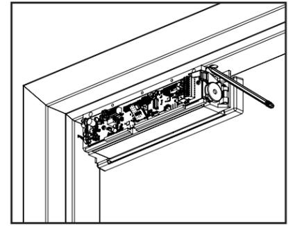
**Diagram 18** Tightening the mounting screws
