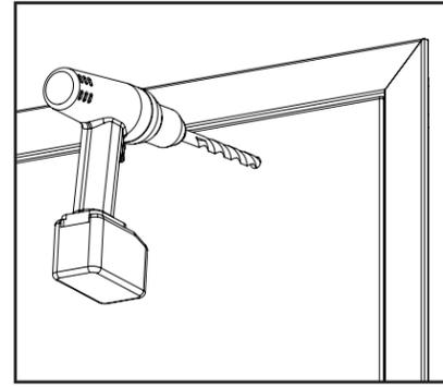
**Diagram 13** Securing the plate assembly to the door
