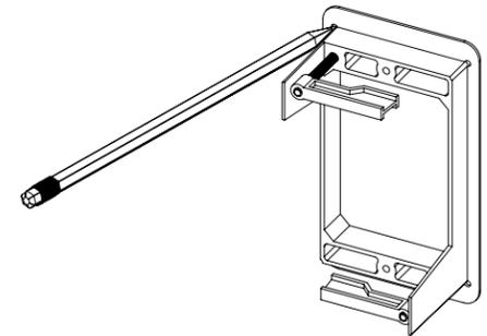
**Diagram 22** Installing the mounting device
