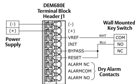
Diagram 27 Typical system wiring with external initiate device
