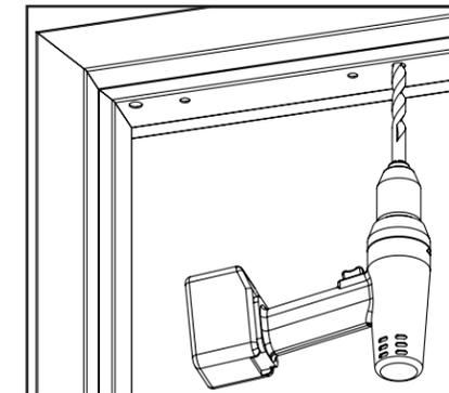
**Diagram 10** Installing the bracket
