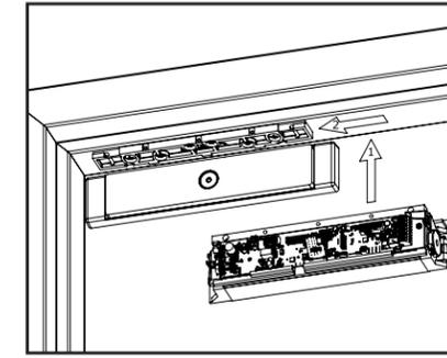
**Diagram 17** Marking the back edge of the mounting bracket
