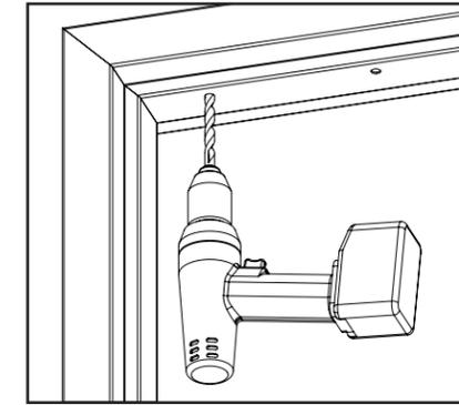
**Diagram 8** Installing the blind nuts
