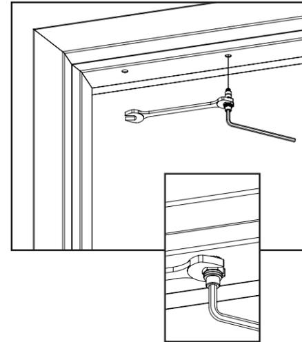
**Diagram 9** Drilling the wire access holes
