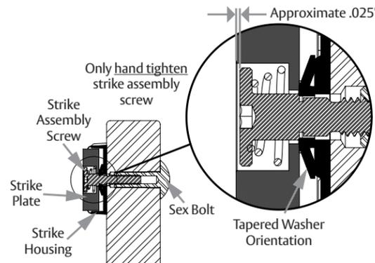
**Diagram 15** Strike assembly installed – inside door
