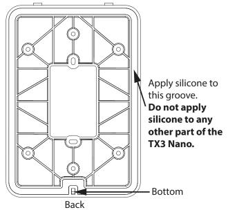
Attach TX3 Nano to mounting plate
