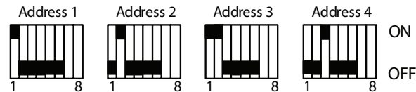
Figure 1: DIP Switch settings for RS-485
