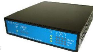
**Technical Considerations** - Before you mount the 5 Port PoE Unmanaged 10/100Mbps Switch/Extender to a fixed location, consider all of the following: Determine optimal placement, check patch cord routing and AC outlet location. Collect and document Network information as required. Ensure the CAT 5 (or higher) cable length from the LP-2334 to the Powered End IP device does not exceed 328 feet/100 meters total length.
