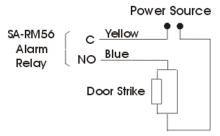
**NOTE:** Power source shall be UL294 Listed Class 2 power-limited, with 4 hours of standby power.
