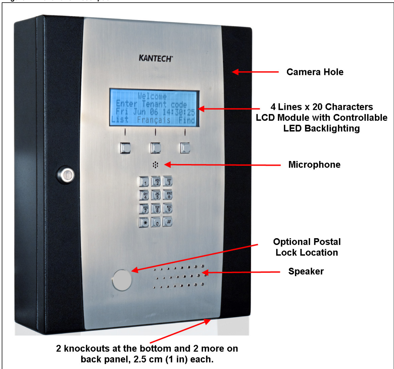
Figure 1: Front Panel Description
