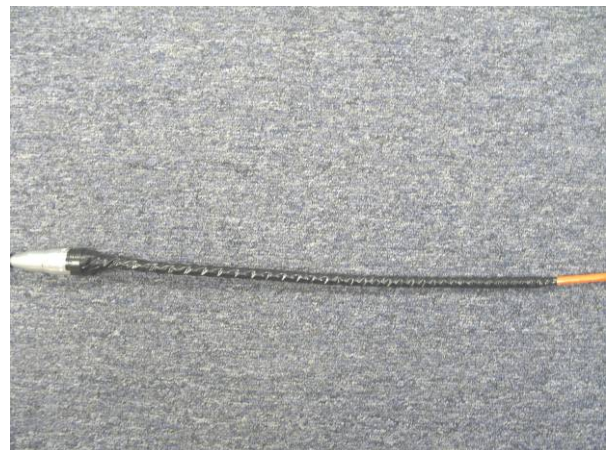
Figure 14: Tape applied over pulling grip
