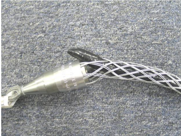
Figure 19: Taped Strength Elements and Buffers Passing Through the End of the Pulling Grip
