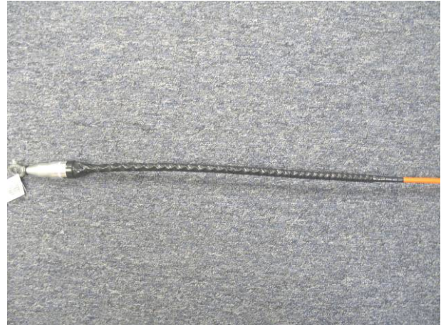
Figure 5: Tape applied over pulling grip
