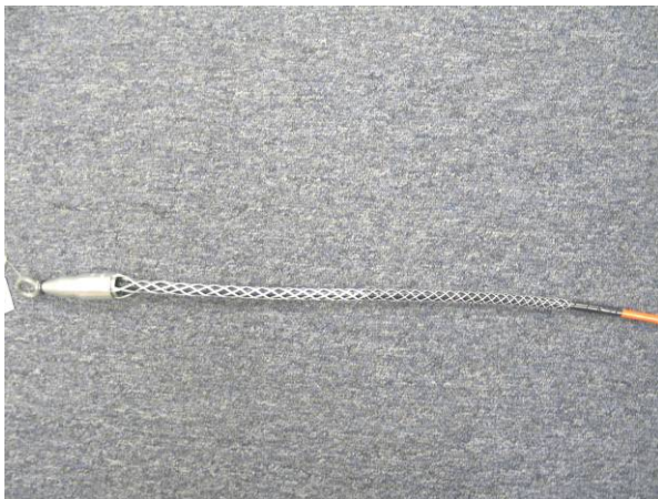
Figure 4: Pulling Grip Installed on Cable
