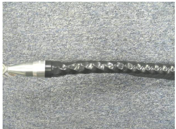
Figure 20: Taped Strength Elements and Buffers Folded Back onto the Grip and Taped
