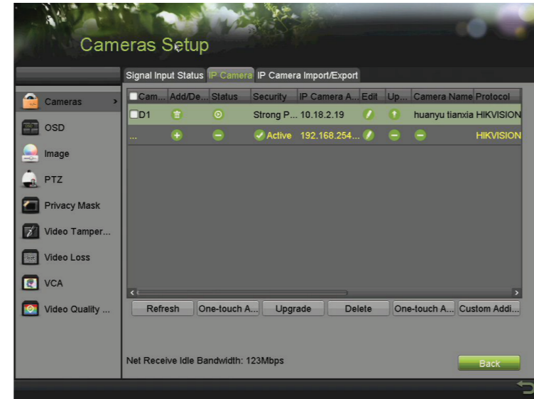
Figure 5, IP Camera Management Interface
