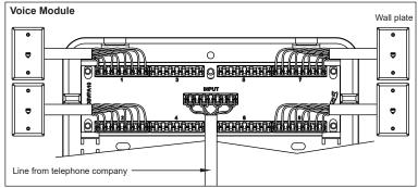
**Step 3a:** Terminate the incoming phone line to the 110 IDC labeled "INPUT". Identify each outlet cable and terminate to 110 IDC labeled "1~8". Note: Line #1= Blue, Line #2=Orange, Line #3=Green, Line #4= Brown.
