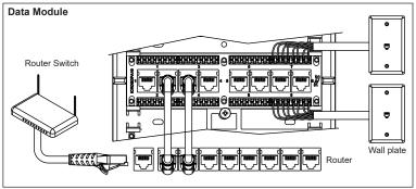
**Step 3b:** Terminate cables on the 4-Pair 110 connectors on the data module. Connect one end of a patch cord to the corresponding jack and the other end to the Ethernet router after identifying the port to activate.
