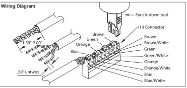
**Step 2:** Terminate the wires by only using a 110 punch-down tool. Be certain to follow the specified T568A color code for 8P8C installations as per TIA-570 residential wiring standards.
