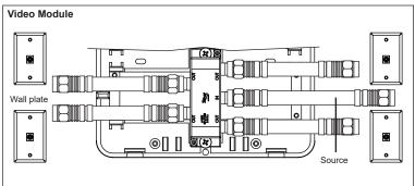
**Step 3c:** Attach a coaxial cable from the antenna or cable TV source to the "IN" connector on the splitter. Up to 4 TV tuners can be connected to the "OUT" connectors.
