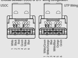
3. Sort wires and place into the IDC.
