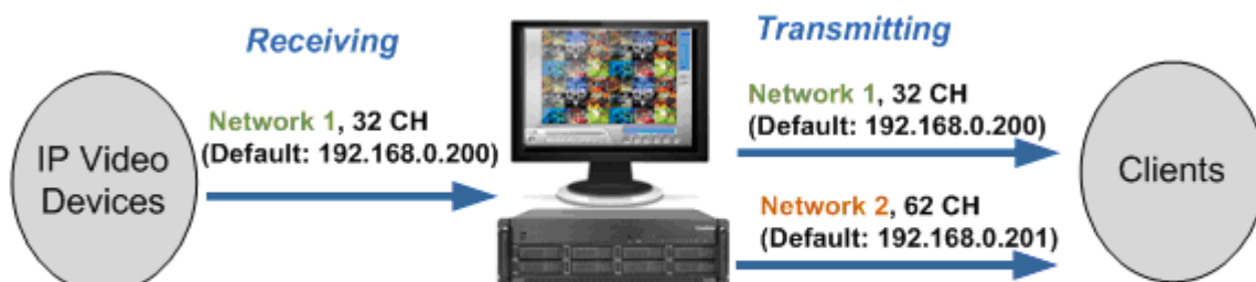
GV-NVRH V5 + 2 Network Cards assigned on different networks
