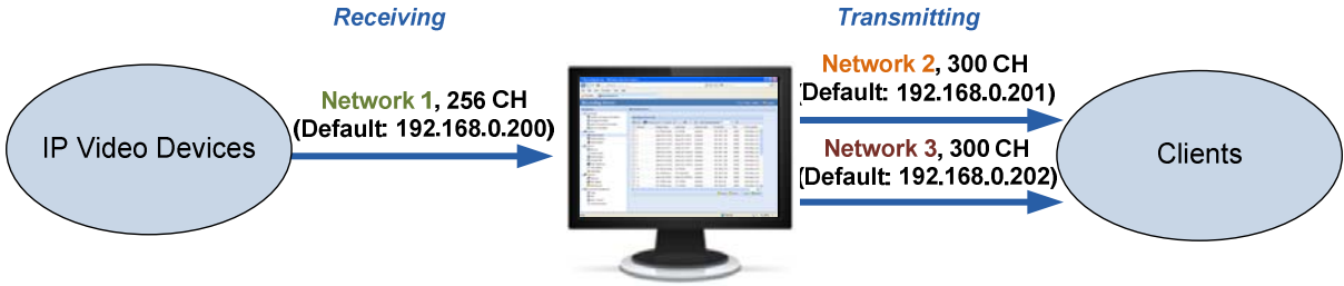
GV-Recording Server + 3 Network Cards assigned on different networks
