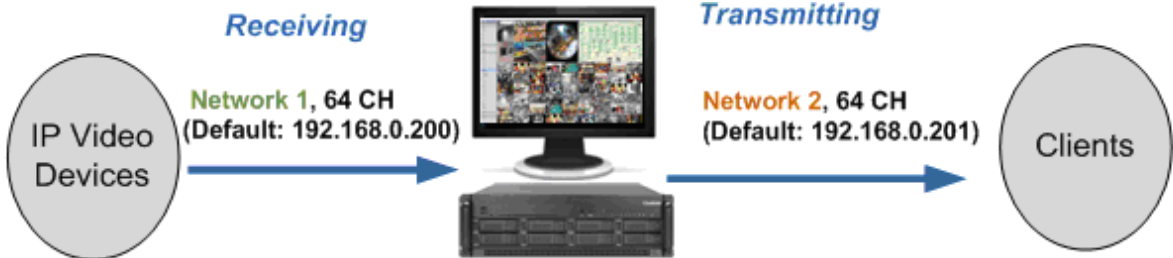
GV-VMSH V5 + 2 Network Cards assigned on different networks
